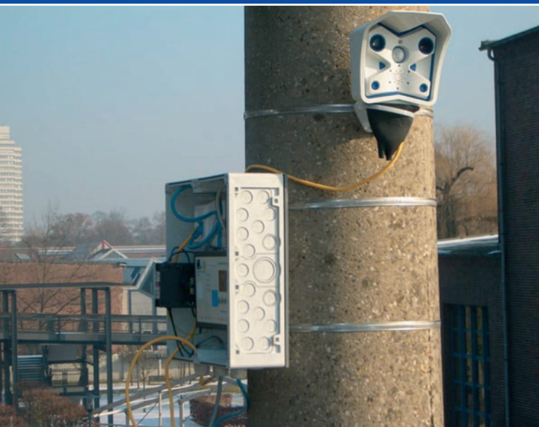
MOBOTIX camera with the (during installation still open) Mobile Connect Box for the UMTS transmission of current traffic images. In the control center (right), this image information is evaluated and any measures required initiated. The traffic monitoring photos shown here are original images captured by the MOBOTIX camera.
